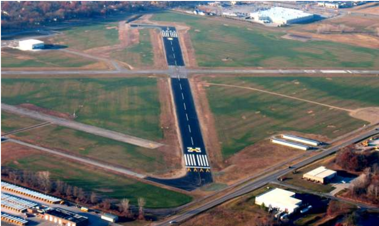
Figure 2-1 Markings for a Temporarily Closed Runway
