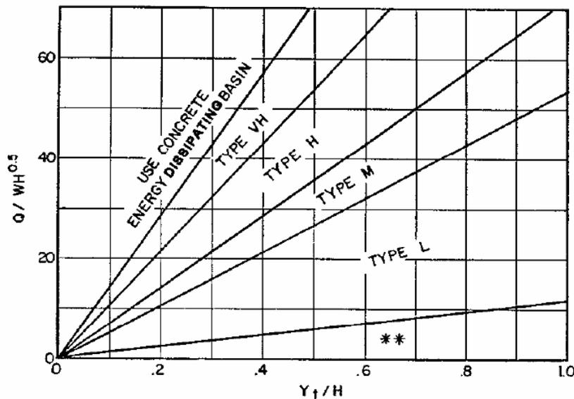
Use  $H_a$  instead of  $H$  whenever culvert has supercritical flow in the barrel.
