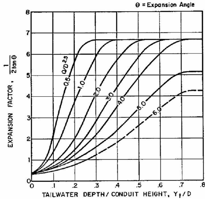
Figure 11.5 Apron expansion factors for rectangular conduits
