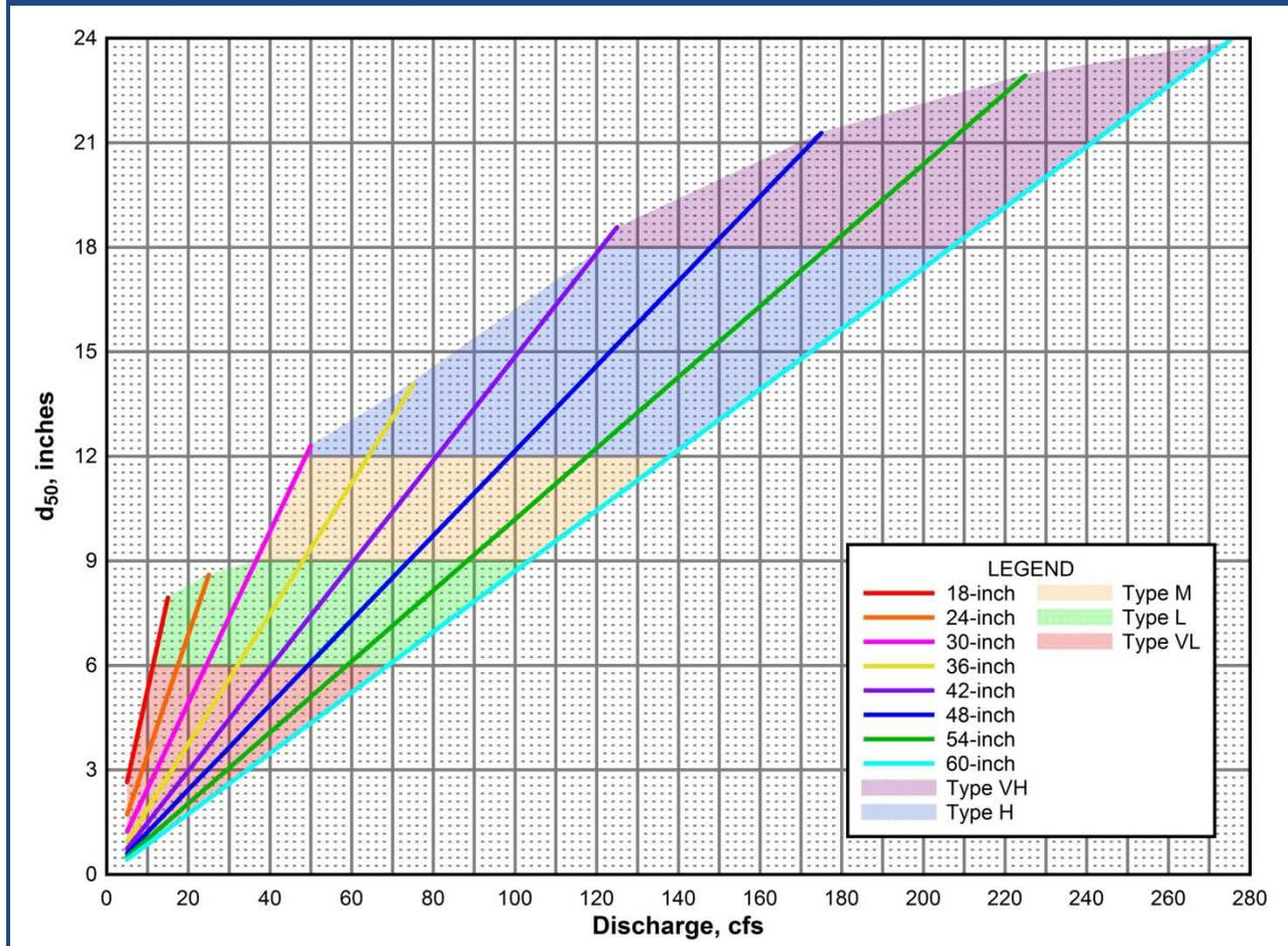
The length (L) from [Figure 11.1](#) of the riprap apron can be estimated using [Figure 11.7](#) or [Figure 11.8](#). These charts correspond with the riprap sizing chart shown on [Figure 11.6](#). Riprap materials shall be in conformance with Section [12.3.5.2](#). Riprap gradations shall conform to [Table 11.5](#). An underlying granular filter blanket, filter fabric, or combination of the two is required for riprap apron installations, in conformance with Chapter 8 of the Hydraulics Manual.
