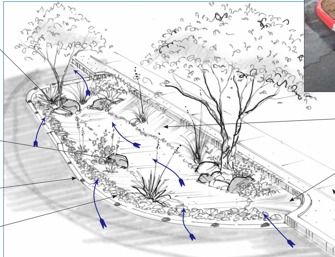
Steeper slopes (up to 50%) are used to maximize area of level bottom 8" deep; all slopes greater than 33% are lined with rock to reduce erosion (rock not shown to reveal basin contours)
