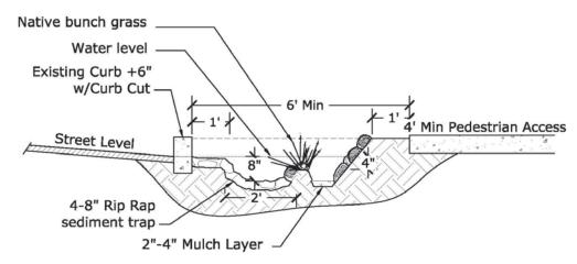
Figure 6. Typical cross sectin of sediment trap for curb cut with rock-lined basin.
