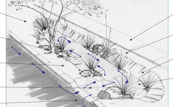
Figure 5. Conceptual drawing of a curb cut and basin with shallow slopes in the ROW.
