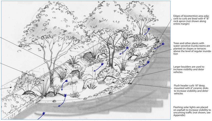
Figure 15. Conceptual drawing of a street width reduction with depressed bioretention area for a neighborhood street.
