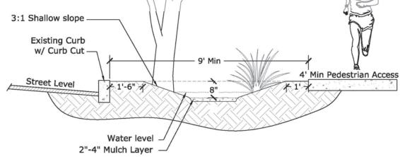
Figure 4. Typical cross-section of a basin with sloping sides, showing typical setbacks for a site on a residential street with on-street parking. For plan view see Appendix.
