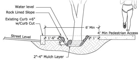
Figure 2. Typical cross-section of a basin with rock-lined edges, showing typical setbacks for a site on a residential street with on-street parking (for plan view see Appendix).
