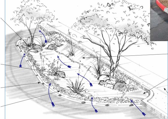
Figure 9. Conceptual drawing of a chicane with bioretention area for a neighborhood street.
