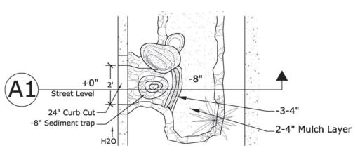
Figure 7. Plan view of sediment trap for curb cut with rock-lined basin.
