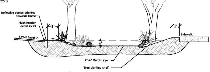
Figure 14. Typical cross-section of a street width reduction with flush curbs and depressed bioretention area. For plan view, see Appendix.
