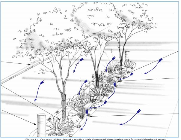
Figure 11. Conceptual drawing of a median with depressed bioretention area for a neighborhood street.
