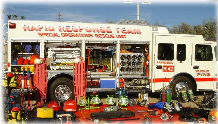
**Special Operations Rescue Unit:** this vehicle carries necessary equipment that supports our special operations teams when they perform: technical rescues, extrication, and water rescue.
