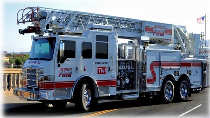
**Quint/Aerial Ladder Truck:** this serves a dual purpose of an engine and a aerial ladder truck. “Quintuple” refers to the five functions that a **quint** provides - pump, water tank, fire hose, aerial device, and ground ladders.
