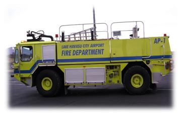
**Airport Rescue & Firefighting Vehicle (ARFF)**: is a type of firefighting apparatus that assists in the emergency response, mitigation, evacuation, and rescue of passengers and crew of aircraft involved in aviation accidents and incidents.
