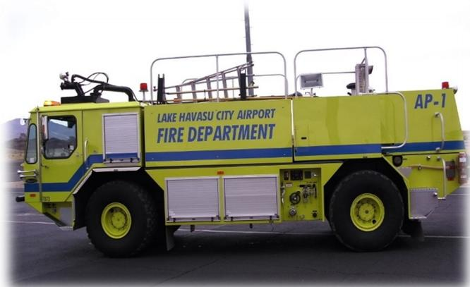
**Airport Rescue & Firefighting Vehicle (ARFF)**: is a type of firefighting apparatus that assists in the emergency response, mitigation, evacuation, and rescue of passengers and crew of aircraft involved in aviation accidents and incidents.
