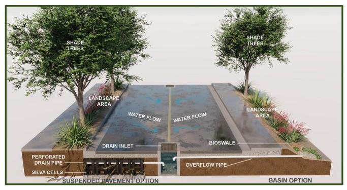
Figure 5-7. Drain inlet capture and distribution example.
