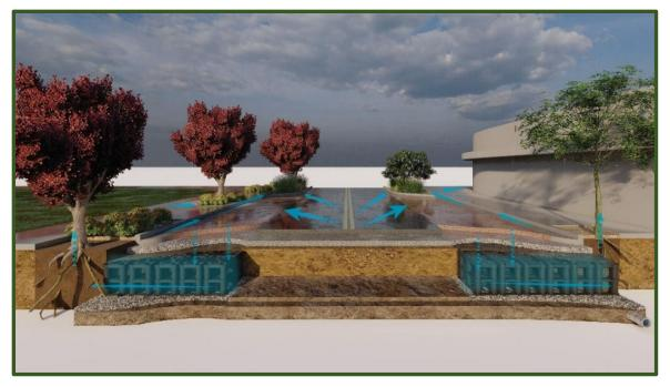
Figure 5-9 Silva Cell water flow diagram. (Lake Havasu City, Author & Source: WERK)
