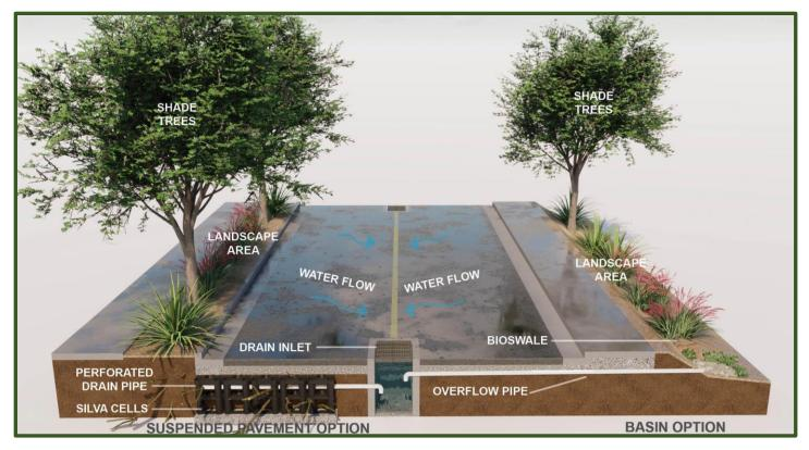
Figure 8-12. Inverted Crown Roadway BMPs – drain inlet capture and distribution to landscape.
