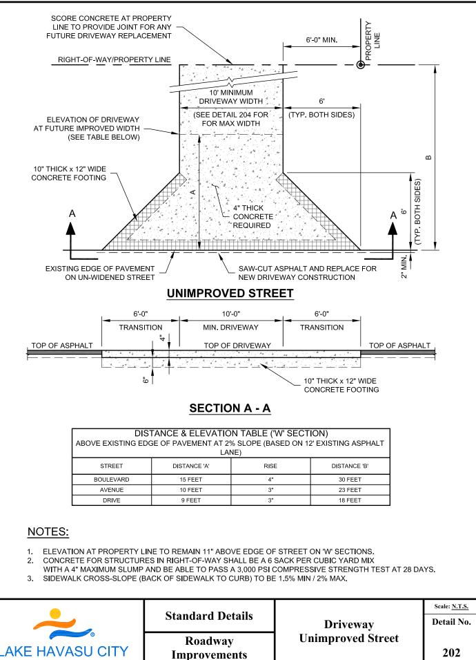
\Lhcdata\engineering\Programs\Standards\Developing Public Works Standards\LHC Standard Details\LHC Series 200 Roadway\DWG\DETAIL 202.dwg
