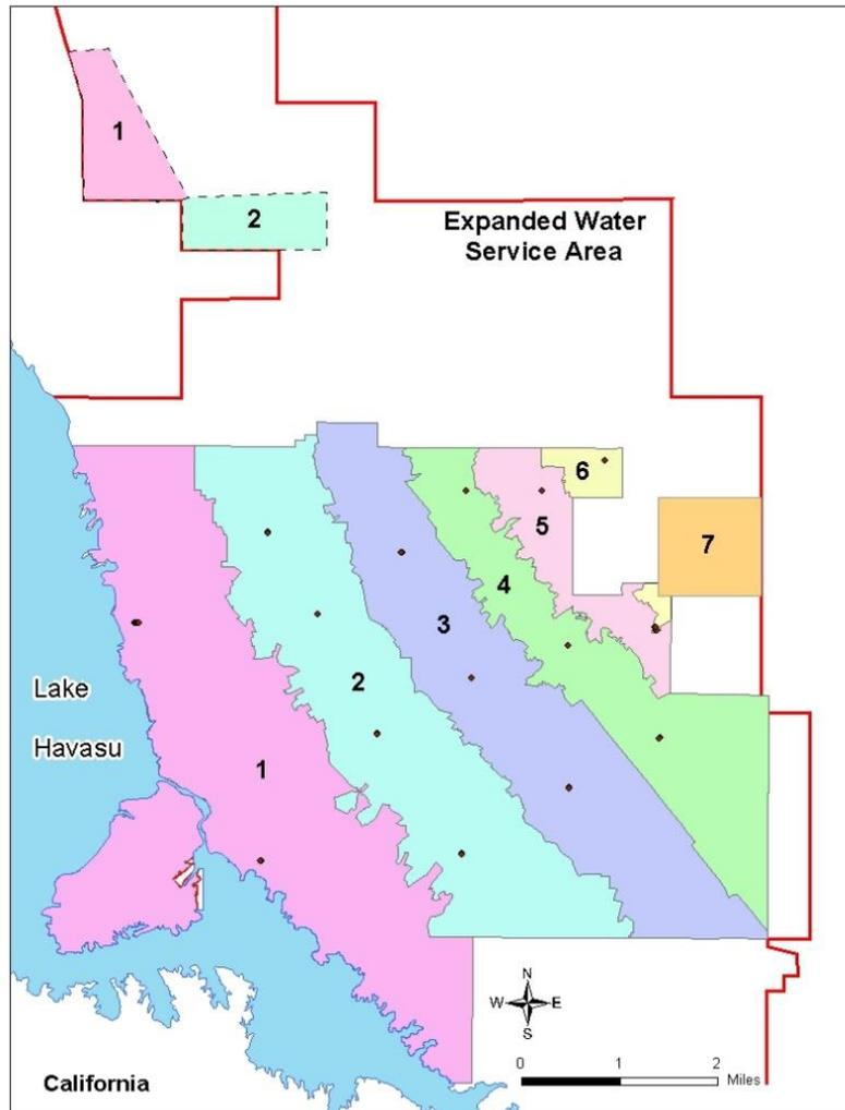
**FIGURE 2-2: WATER PRESSURE ZONES (1-7) AND PUMP STATIONS (DOTS) IN LAKE HAVASU CITY FOR WATER DISTRIBUTION REFLECTING THE CITY'S 2-4° SOUTHWEST SLOPING TOPOGRAPHY**
